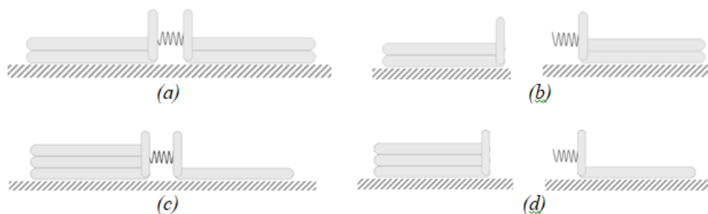
Fig 6. Objects to draw forces interaction diagram: (a) two same-mass sleds before the launch; (b) two same-mass sleds after the launch; (c) two different-mass sleds before the launch; (d) two different-mass sleds after the launch
