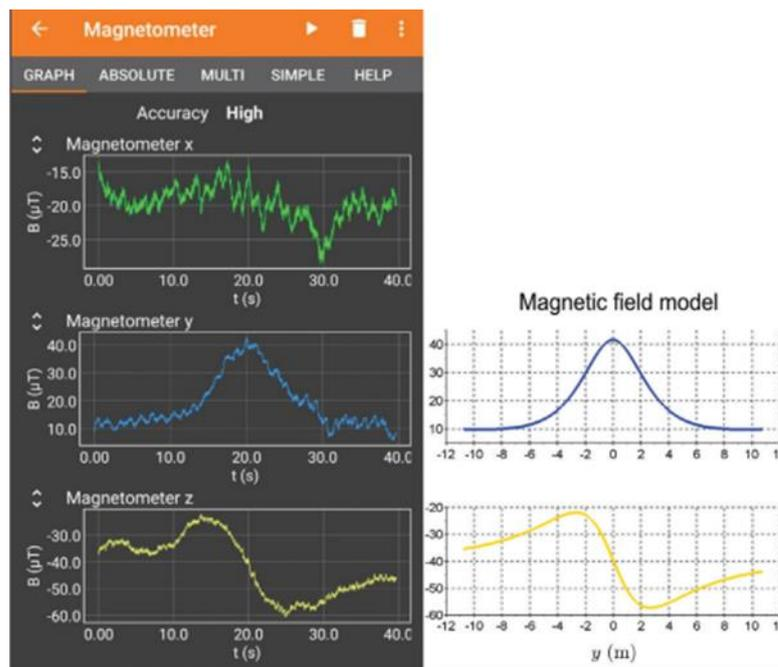
**Fig 3.** Comparison between the measurements and the model calculation [25]
