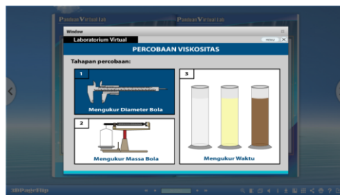
Figure 3. Measurement of diameter, mass and time in a viscosity experiment
